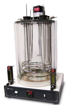
K43041 Sequence IV Liquid Foaming Characteristics Apparatus
