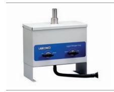
7394800 - Liquid Nitrogen Secondary Trap. For samples with ultra low eutectic points. Liquid nitrogen cools to -196° C (-321° F) to trap contaminants. Powder-coated steel. 3/4" OD inlet and outlet connections. Includes insulated filler tube for connection of user-supplied liquid nitrogen tank, 20" wire-reinforced PVC tubing, 3/4" ID and two clamps. Liquid nitrogen is required (not included). Shipping weight 24 lbs. (11 kg) △ WARNING: Cancer – P65Warnings.ca.gov (California only)
