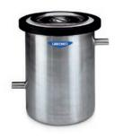
7538000 - Dry Ice Secondary Trap. For samples with low eutectic points. Dry ice and solvent cools the insulated well to approximately -75° C (-103° F). When used alone, it may serve as an inexpensive collector. Connect a sample directly to the incoming port and add a vacuum pump to the outgoing port. Ice trapping capacity of 900 ml. Includes 3.1 L well and 3/4" OD inlet and outlet connections. Dry ice and solvent, such as alcohol, are required (not included). Shipping weight 9.0 lbs. (4.1 kg)
