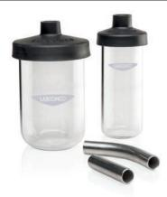
**7540100—FreeZone Freeze Dry Glassware Kit.** Includes one each flask and adapters: 7540800 (600 ml) and 7540600 (300 ml), 7547200 (3/4" straight stainless steel) and 7547600 (3/4"  $45^{\circ}$  bend stainless steel). Shipping weight 5.0 lbs. (2.0 kg)
