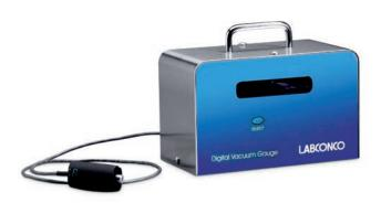
Digital Electronic Vacuum Gauges. LCD displays vacuum measurement in mBar, Torr or Pa. Range is 0.02 to 5 mBar. Stainless steel and powder-coated steel casing. 8.1" w x 4.1" d x 6.4" h. Include a cord with 3/8" to 1/2" OD adapter for connection to either vacuum tubing or a valve on a drying accessory. May be used as an accessory by the Dry Ice Benchtop Freeze Dryer or other freeze dryers. For use with Dry Ice Benchtop Freeze Dryer. Shipping weight 10 lbs. (5 kg)
