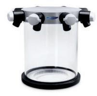
Clear Chambers with Valves. For interior view of product shelves and glassware connection. Includes acrylic base, anodized aluminum lid, and eight neoprene valves with molded plastic knobs. For 1/2" and 3/4" flask adapters. 8" dia. opening and cap for 3" dia. attachment port.
