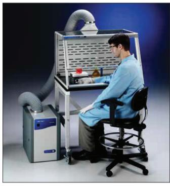
For light duty applications, Protector XVS Ventilation Stations may be paired with FilterMate Portable Exhausters, which return filtered air to the laboratory.
