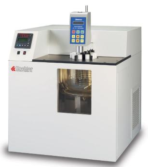
K34715 Programmable Brookfield Viscosity Liquid Bath System (BVS5000)
