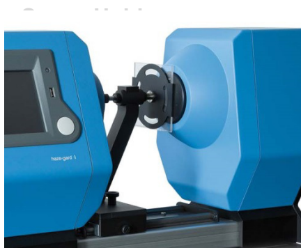
The measurement of haze is used to determine abrasion resistance of transparent materials. The haze-gard i Abrasion Holder facilitates positioning of the abraded area in the measurement beam.
