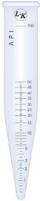
"Finger Tubes" Finger tubes have a 12.5ml capacity. ASTM D96 or D4007
