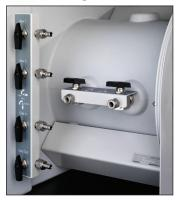
Includes six each manual ball valves, pressure relief valve, compression fittings, hose connector fittings, holesaws, O-rings and nuts to add four service valves to the main chamber and two service valves to the transfer chamber. Two of the valves on the main chamber and two on the transfer chamber may be used for evacuating and filling. The remaining two on the main chamber are for drying train connections. Requires installation. Precise Controlled Atmosphere Glove Boxes include six manual
