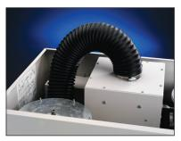
Changes the builtin blower operation from standard negative pressure to positive pressure operation. The blower pushes instead of pulls HEPA filtered air through the main chamber. Typical applications for positive
