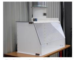
The Powered Exhaust Hood with Inline Fan pulls most of the harmful fumes away from the operator's breathing zone (40" pictured above & below).
