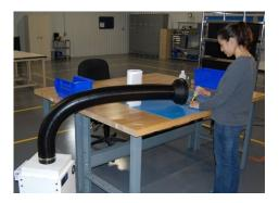
Model 300 Floor Sentry can be used to extract fumes from a wide variety of applications.
