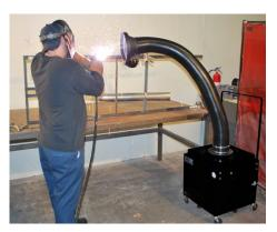
The Model 400/450 Portable Floor Sentry helps protect the operator from fumes by extracting at the source.
