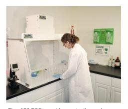
The 48" PCR provides a sterile workspace for a variety of medical applications (Single air cleaner unit shown above).
