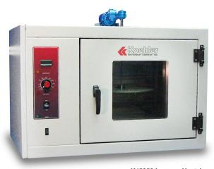
K45850 Loss on Heat / Thin Film Oven
